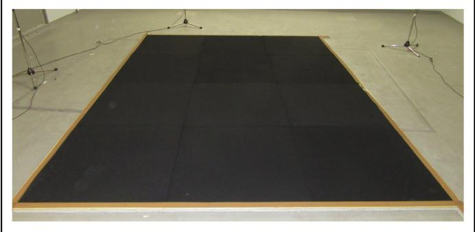
Picture of the test setups in the reverberation room. top: sheets with 15 mm thickness (version 1) bottom: sheets with 25 mm thickness (version 2)
